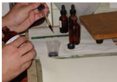
Step 4: An equal measurement of palladium and platinum solution is added to the ferric oxalate mixture to create the sensitizer.
