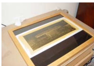
Step 11: The negative and coated paper are placed in a contact printing frame to create even pressure between the negative and coated paper.
