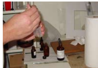
Step 3: The specified amount of ferric oxalate chemicals are measured out using eyedroppers in a small medicine cup.
