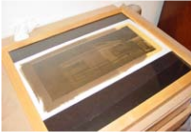
Step 13: The undeveloped test strip after exposure. Darkest area = longest exposure time. Lightest area = shortest exposure time
