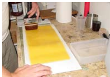
Step 8: All puddles and bubbles are smoothed out and the coated area is as even as possible.
