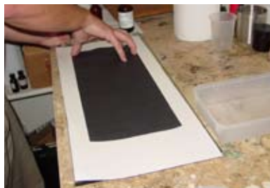
Step 2: a scrap sheet of paper the same size of the negative is laid out to mark the size and area to be coated.
