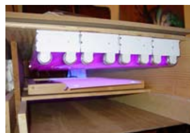
Step 12: The coated sheet is exposed to UV light in an exposure unit with 8 blacklight fluorescent tubes. For a specified amount of time.
