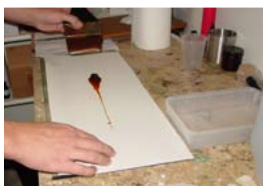
Step 5: The sensitizer solution is quickly poured out along the length of the paper.
